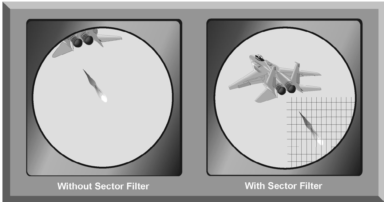
Figure 14-19. Sector Attenuation “Response” Technique
