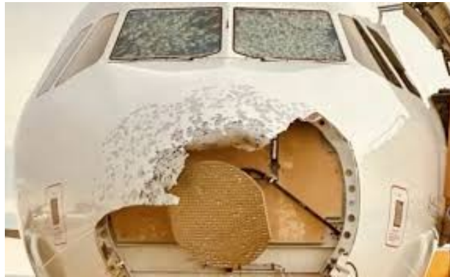
FIG. 3. Austrian Airlines Mayday after severe hail damage [5]
