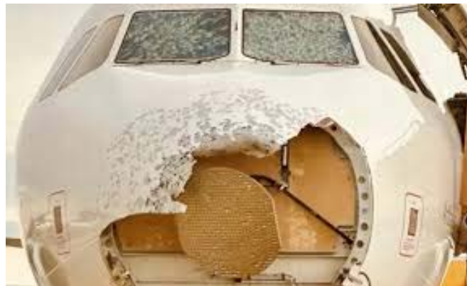
FIG. 3. Austrian Airlines Mayday after severe hail damage [5]
