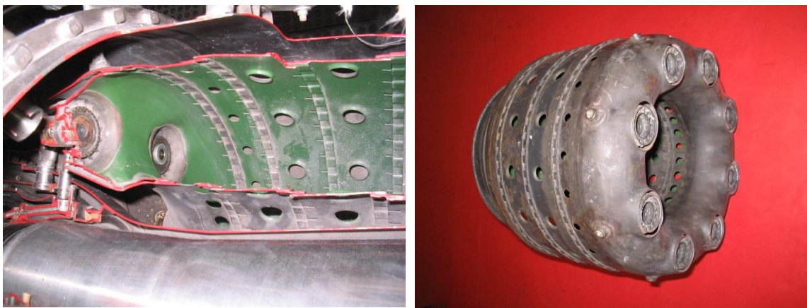
FIG. 4. To the left annular combustor, to the right an annular liner [own photo]
