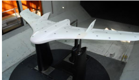
FIG. 3 Model mounted on the balance inside the subsonic wind tunnel
