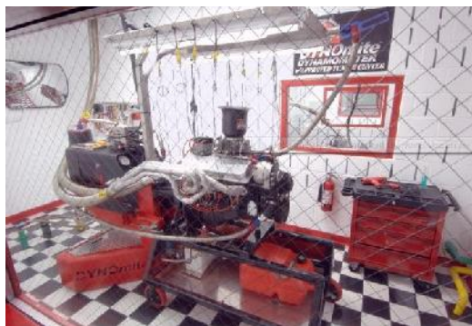
(a) Stationary Test Stand Dynos
