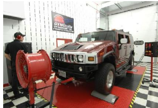
(b) single-axle, dual-axle, and even AWD tri-axle dynos
