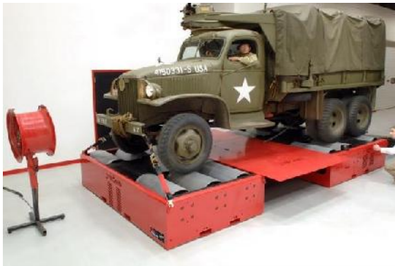
(a) heavy-duty (20”roll) AWD systems for multi-axle trucks
