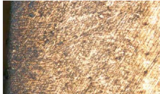
FIG. 4. 41Cr4 improved steel and superficial hardened with electron beam. Nital Attack 200:1
