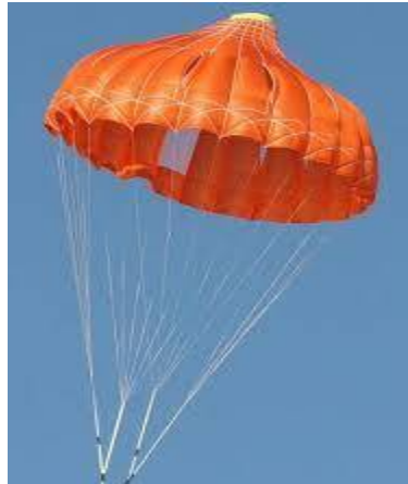
FIG. 2 Rescue parachute PL-70
