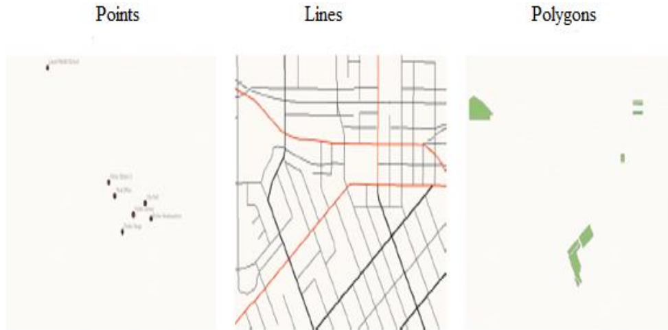
FIG.5. Creating points for locations, networks of streets and parks limits are examples of feature class [8.10]
