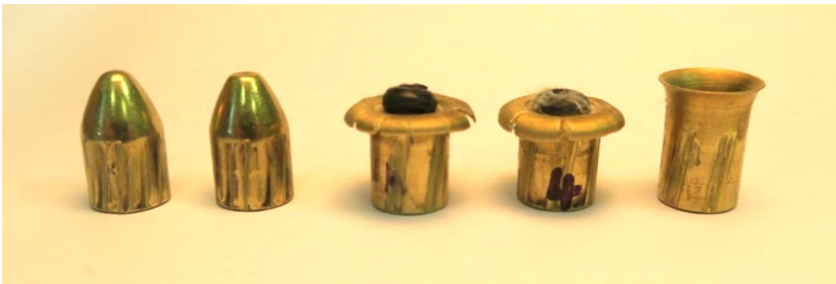
Figure 3. Deformation of projectiles (1. FMJ water, 2. FMJ 75 starch, 3. A5 75 starch 4. A5 honey ,5. A5 water)
