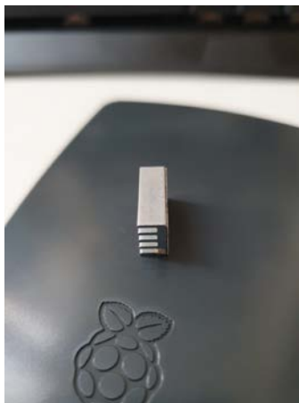
Fig. 3 The original plastic case with radiators that you stick with double-sided adhesive tape on the hotspots of the Pi board (CPU, USB Controller and RAM).
