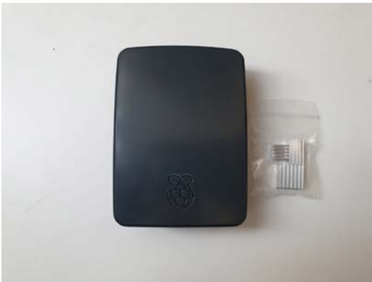
Fig. 3 The original plastic case with radiators that you stick with double-sided adhesive tape on the hotspots of the Pi board (CPU, USB Controller and RAM).
