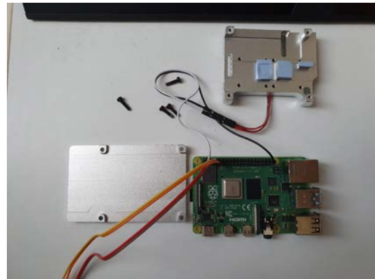
Fig. 5 The aluminum case with thermal pads placed on the hotspots
