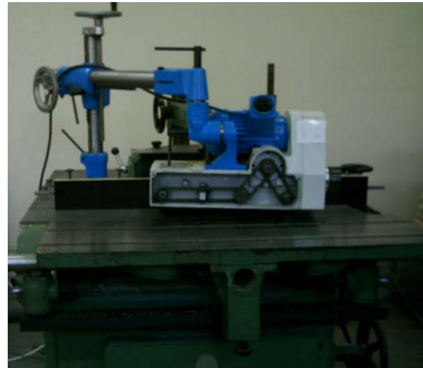
Fig. 3. Vertical milling machine type MNF10 with mechanical feed device.
