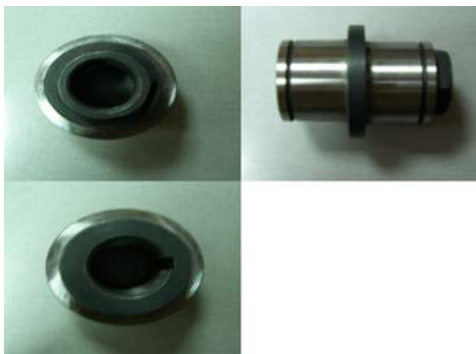
Photo 4. Main component eccentric bushing device from the superfinishing tools provided with hard-alloy glued plates.
