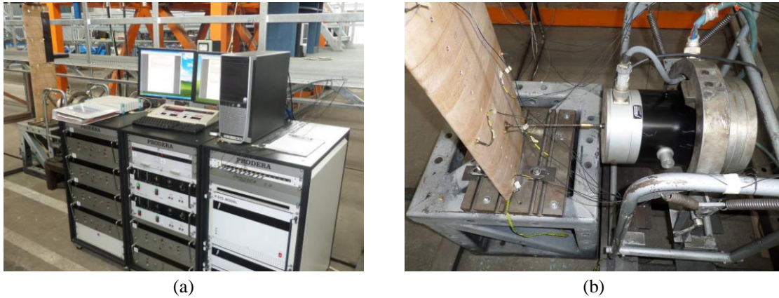
FIG. 1. (a) Prodera equipment, (b) Mechanical link between exciter and wing structure
