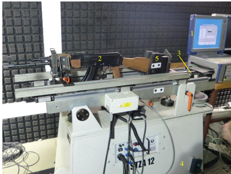
FIG. 4. View of the experimental setup: 1 – ballistic computer, 2 – AK 47 rifle with tubeless recoil system inside, 3 – piezoelectric force sensor, 4 – mobile firing rest, 5 – elastic stay.
