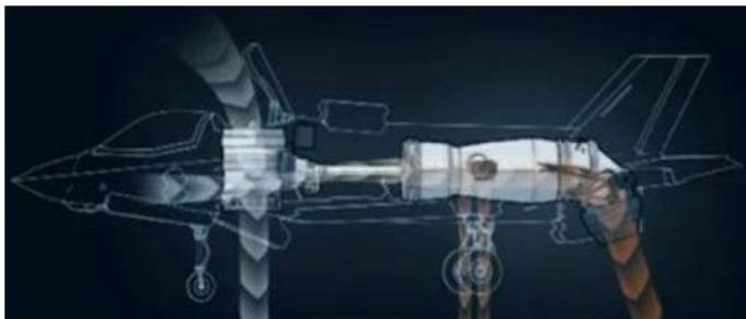
FIG. 3 Vectored thrust obtained by steering nozzle
