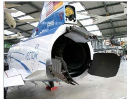
FIG. 4 Vectored thrust obtained with deflection shutter
