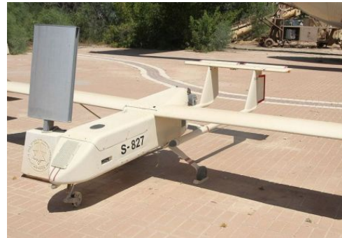
FIG. 2.7. Tadiran Electronic Systems Mastiff , [15]
