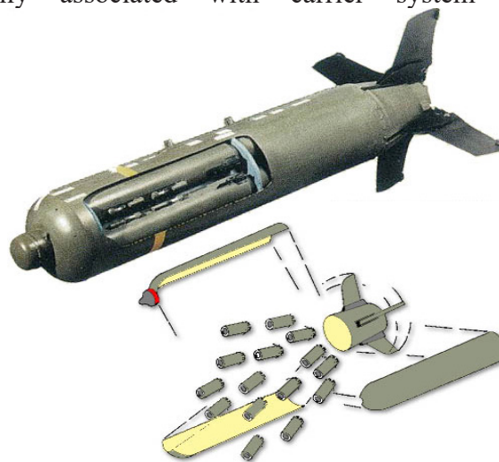
Fig. 5 The carrier system CBU-97 (Source: defense industry daily, [8])
